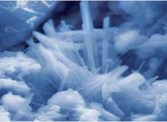
PENETRON active ingredients react with concrete minerals to form insoluble crystals, which fill in cracks, pores and voids up to a width of 400 microns (0.4 mm). (Magnification 5,000x)
